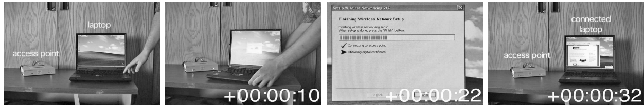
Figure 1. Connecting a laptop to a secured wireless network in 32 seconds. All the user has to do is briefly align the infrared ports of laptop and access point and press the Enter key twice. These are snapshots from a live Network-in-a-Box demonstration.
