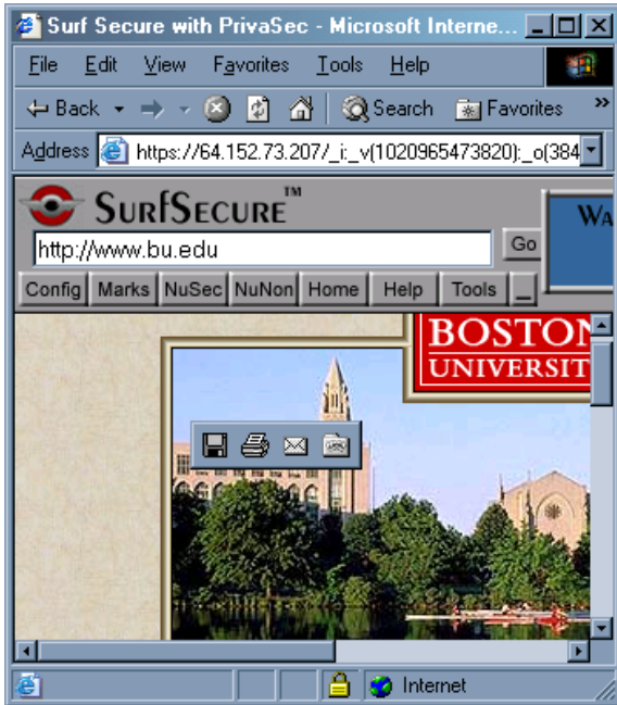
Figure 4: PrivaSec screen shot showing SafeWeb technology. The top frame is a control panel (“SurfSecure”), and the bottom frame is the page requested by the user.
