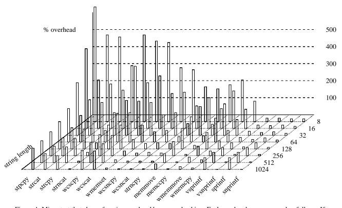
Figure 4: Micro test that shows function overhead by range checking. Each overhead was measured as follows; If an intercepted function is 2.5 times slower then the overhead is 150 percent ( $(2.5-1) \times 100$ ).
