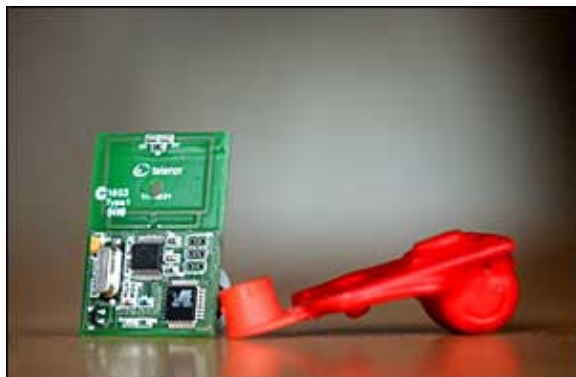
Figure 5: The radio tag, ordinary version to the left and a packed version to the right, ready to be mounted in the ear of the sheep.
