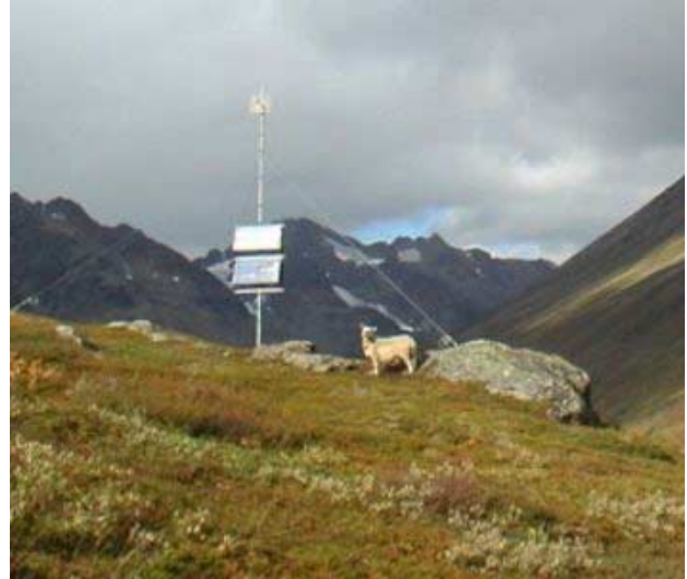
Figure 10: Fixed access point and a sheep with radio tag in the test field.
