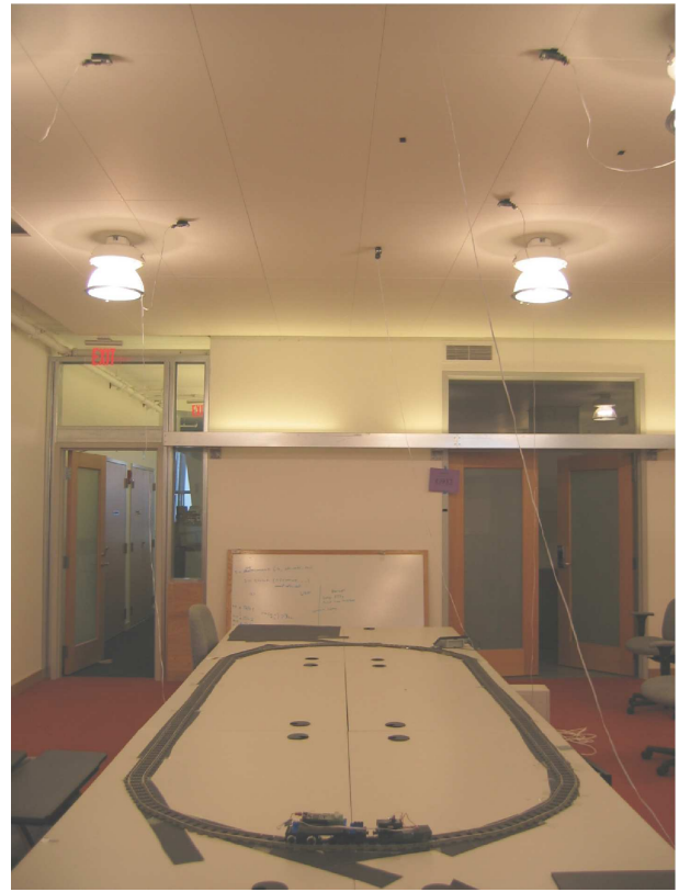
Figure 5: Picture of the experimental setup. The beacons are shown on the ceiling; the cables emanating from the beacons are used in a subset of the active mobile experiments to report distance samples observed by infrastructure nodes.
