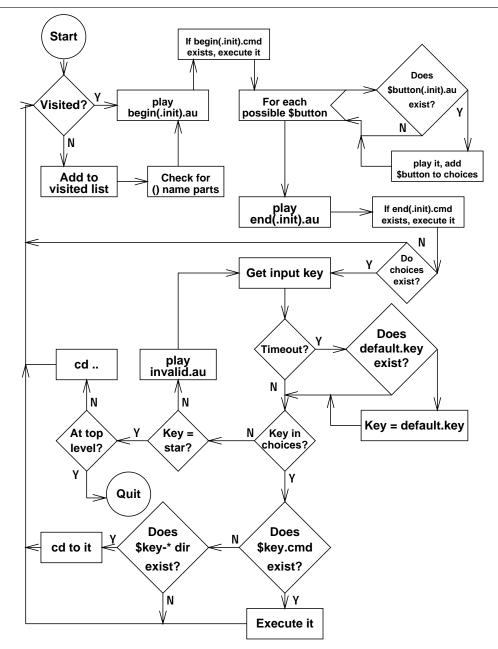
Figure 3: Tree processing algorithm.
