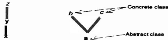
Two class hierarchies in the message passing system, with abstract classes a,x and concrete classes z,b,c
