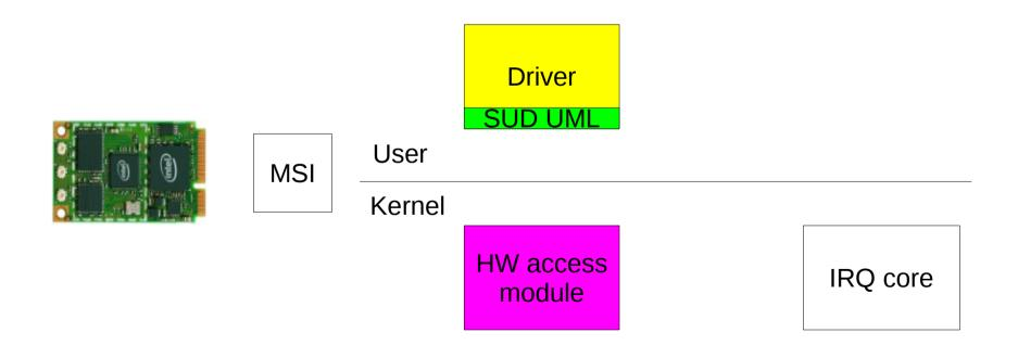
Kernel calls HW access module interrupt handler HW access module masks interrupt with MSI
