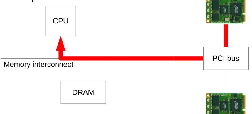
Driver configures the device to execute attacks DMA to DRAM Peer-to-peer messages Interrupt storms
