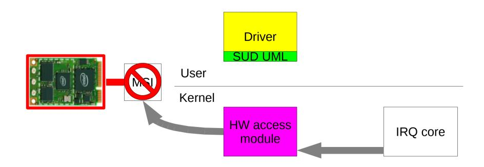
Kernel calls HW access module interrupt handler HW access module masks interrupt with MSI Asynchronous RPC to driver
