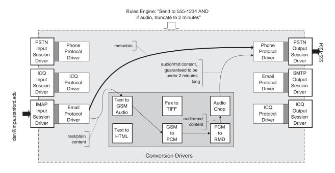
Figure 5: The Dispatcher. This figure shows how the Dispatcher routes email arriving at the Personal Proxy's email address to the telephone number at which Dan can be presently reached. Thin light arrows indicate content flow. Thin bold arrows indicate metadata flow.
