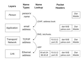
Figure 1: The Layering Model. We show the traditional networking layers, extended with the *Person* layer. *Name Types* shows examples of the kinds of names used at each layer. *Name Lookup* shows some methods of mapping names from each layer to names in the next lower layer. *Packet Headers* shows examples of actual names at each layer, and their relative locations in a typical email packet.
