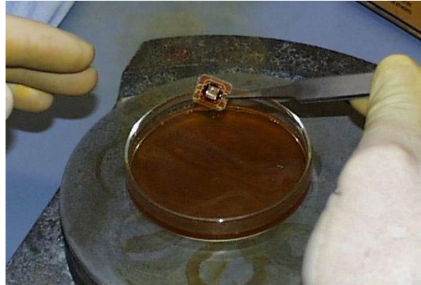
Figure 1: Hot fuming nitric acid (> 98% \text{HNO}_3 ) dissolves the package without affecting the chip.
