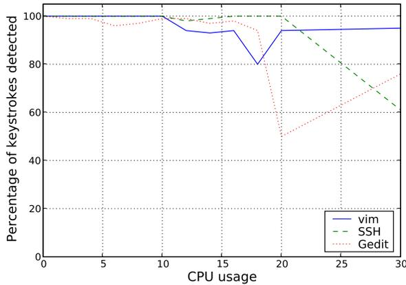
Figure 7: Percentage of keystrokes detected vs. CPU usage
