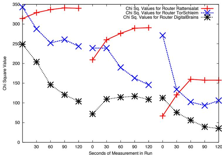
Figure 8: This graph shows three sets of cumulative  $\chi^2$  computations for three nodes; the actual entry node (Rattensalat), a node that initially shows up as a false-positive (TorSchleim) and a typical negative (DigitalBrains). As expected, the  $\chi^2$  values (at time 120 s) are consistently the highest for the correct node; false-positives can be ruled out through repeated measurements.
