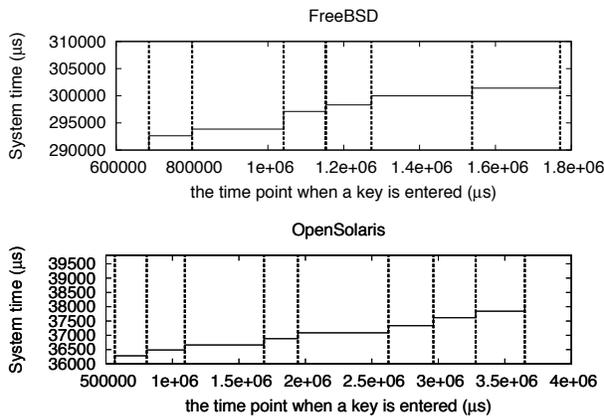
Figure 11: System time (solid line) vs. keystroke events (dashed line) in `vim` under FreeBSD (Release 7.1) and OpenSolaris (Release 2008.11). In the experiments, we found that the system time of `vim` changed only in response to keystrokes, which were recorded by shadow programs.
