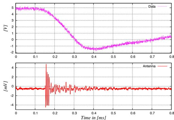
Figure 4: A falling edge of the data signal (upper graph) and the electromagnetic emanation of the keyboard (lower graph). The compromising emission is not directly generated by the data signal such as described by Smulders in [30].
