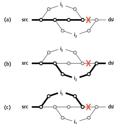
Figure 6: **Disjoint paths.** (a) The default path to the destination fails due to a faulty link. (b) Routing through intermediary *i*<sub>2</sub> would succeed, since the diverted path is disjoint from the faulty link. (c) Routing through intermediary *i*<sub>1</sub> would fail, since the diverted path rejoins the default path before the faulty link.
