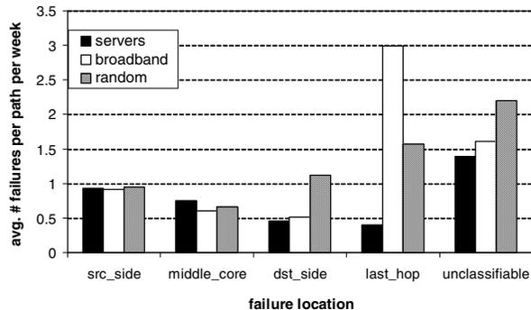
Figure 2: **Location of failures.** Failures are spread throughout the Internet for all three destination sets. Last-hop failures dominate other failures for broadband hosts, but for popular servers, last-hop failures are rare.
