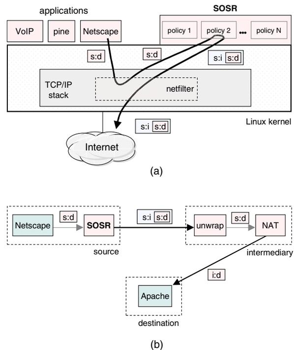
Figure 15: **The SOSR architecture.** (a) The source node uses netfilter to redirect packets from the Linux kernel to a user-level SOSR policy module, which encapsulates the application packet and tunnels it to a chosen intermediary. Note that the application is unmodified. (b) The intermediary node decapsulates the packet, passes it through a user-level NAT daemon, and transmits it to the (unmodified) destination node.
