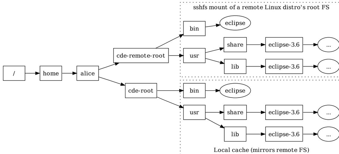
Figure 9: An example use of CDE’s streaming mode to run Eclipse 3.6 on any Linux machine without installation. `cde-exec` fetches all dependencies on-demand from a remote Linux distro and stores them in a local cache.
