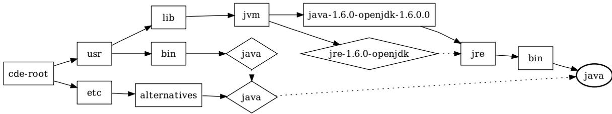
Figure 7: The result of using OKAPI to deep-copy a single `/usr/bin/java` file into `cde-root/`, preserving the exact symlink structure from the original directory tree. Boxes are directories (solid arrows point to their contents), diamonds are symlinks (dashed arrows point to their targets), and the bold ellipse is the actual `java` executable file.
