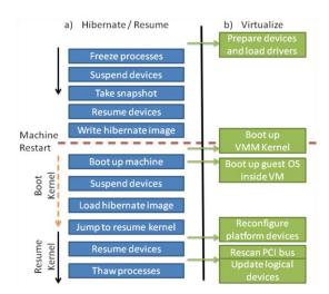
Figure 2: Comparison between the hibernate/resume process and the virtualize process.
