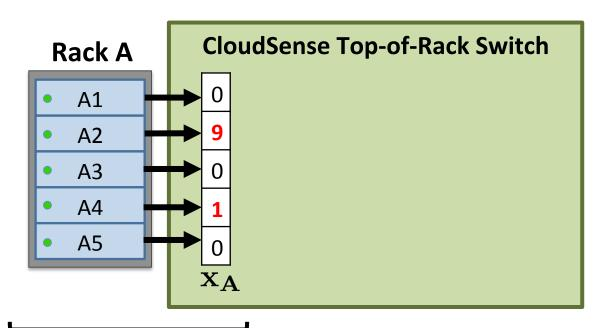
Step 1: Collect Switch collects status of each node (N=5) into a signal vector  $\mathbf{X}_A$ .
