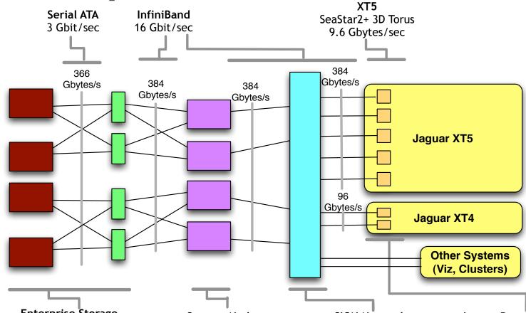
**Enterprise Storage** controllers and large racks of disks are connected via InfiniBand.
