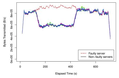
Packet-loss fault may also deviate network throughput
