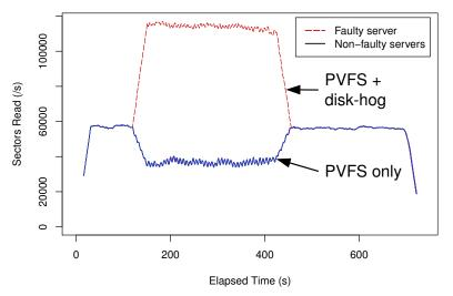
Throughput diverges due to disk-hog on faulty server
