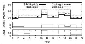
Figure 11: Power consumption, remap operations, and aggregate load across time for a single day.
