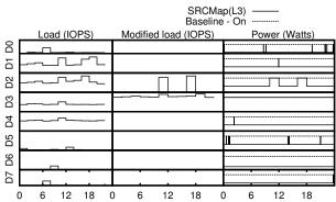
Figure 12: Load and power consumption for each disk. *Y* ranges for all loads is [1 : 130] *IOPS in log-*arithmic scale. *Y* ranges for power is [0 : 19] *W*.
