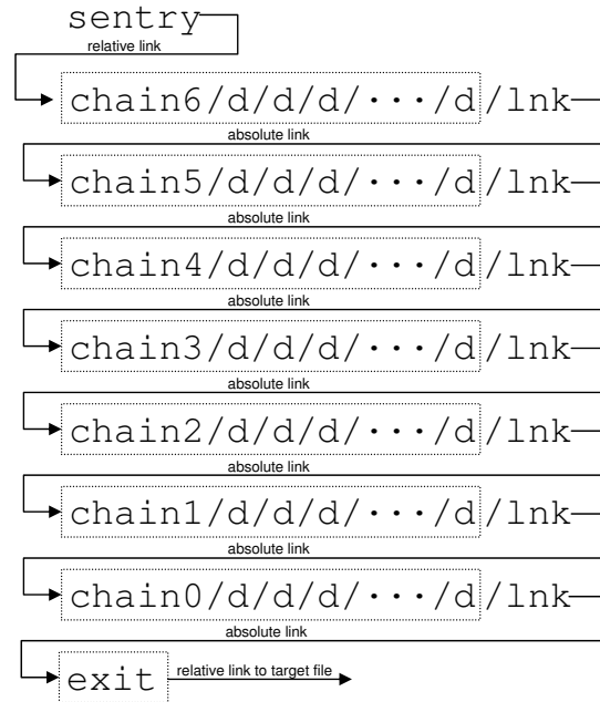
Figure 4: The structure of a six-chains filesystem maze. Arrows represents symbolic links. (Originally published in [5]; reprinted with permission.)
