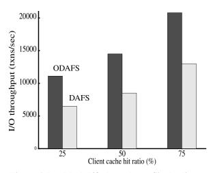
Figure 6. PostMark I/O throughput. Single client with variable cache hit ratio.
