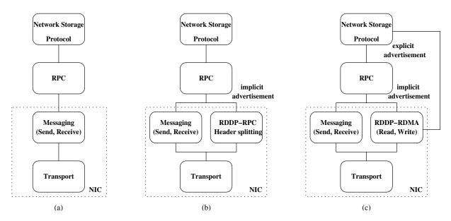
Figure 1. Protocol stack with the messaging and transport protocols offloaded to the NIC (a). RDDP is possible either by separating the data payload when in-lined in the RPC (b) or with RDMA (c).
