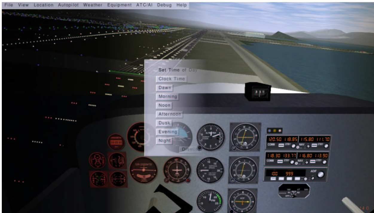
Figure 1: Pilot’s view from a Cessna 172 making a poor approach for landing at San Francisco International Airport. The “Time of Day” pop up menu is partially visible, with seven quick selects and an additional button for typing in the time. Seven consecutive screen dumps, from a wide screen display, have been combined to demonstrate the simulator’s lighting model
