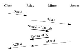
Figure 12 An incorrectly clustered client to server write
