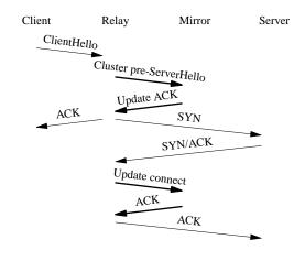
Figure 22 Parallel client and server handshakes
