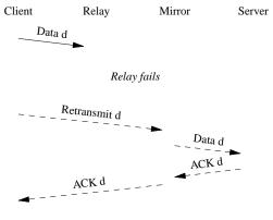
Figure 9 Failure after first data write
