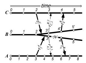
Figure 4: An example showing a dishonest service B that maintains two timelines, entangling one with A and another with C. Event  $\mathcal N$  is committed on the bottom branch of B's timeline, but does not appear on the top branch.
