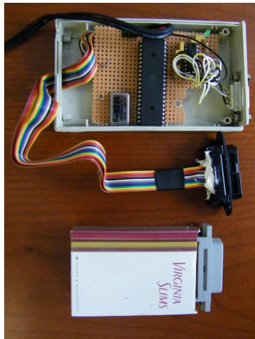
Top left: Cartridge reader/writer prototyped by Hovav Shacham’s research group [7]. Bottom left: Our nonfunctional mockup of installation in cigarette pack. Right: “Gumstix” computer that could be programmed to alter votes in cartridge.
