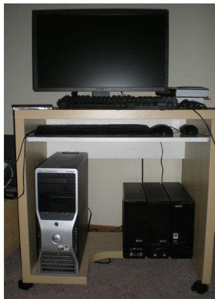
FIGURE 2. HYDRA, A MINIATURE CLUSTER WITH ONE MASTER PC AND THREE NODES, IS THE FIRST AUTHOR'S PRIVATE CLUSTER FOR HOME OFFICE USE. THIS IS ONE OF A SERIES OF INSTALLATIONS OF VARYING SIZES WE HAVE BEEN WORKING ON.
