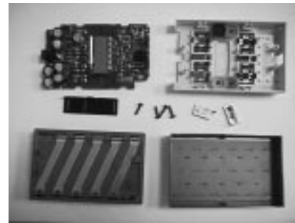
Figure 1: The Lego RCX, opened [12]
