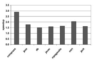
Figure 9: Benchmark speedup when enabling register allocation. The performance number represents the ratio between the measured runtime with the nonoptimized compiler and the optimized compiler running register allocation only.
