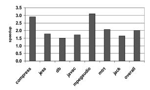
Figure 13: Benchmark speedup of optimized version using register allocation, floating-point optimization, and method inlining compared to the non-optimized implementation of the FastVM on x86.
