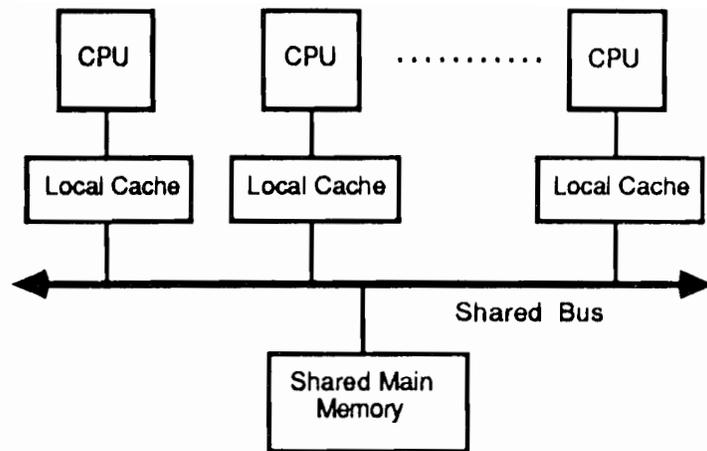
Figure 1. Machine model used in the simulation.
