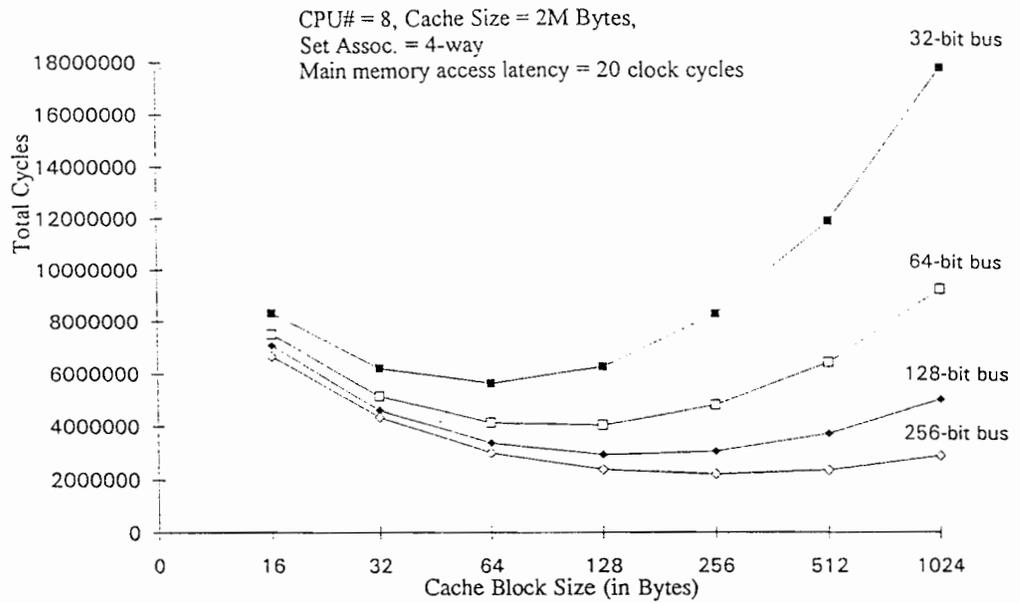
Figure 3. Bus traffic versus block size in systems that have 8 CPUs, 2-megabyte 4-way set-associative caches, and a main memory with a latency of 20 clock cycles.
