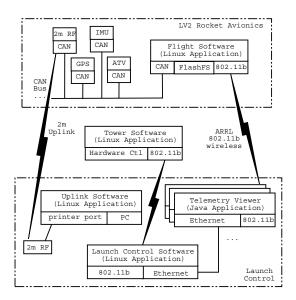
Figure 1: LV2 System Software
