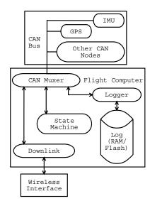
Figure 2: Muxer Flight Computer Software Design
