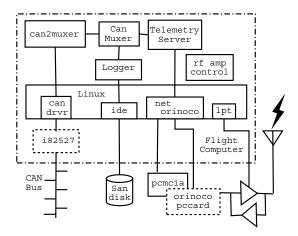
Figure 3: Renegade Flight Computer Software Design
