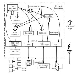
Figure 4: FCFIFO Flight Computer Software Design
