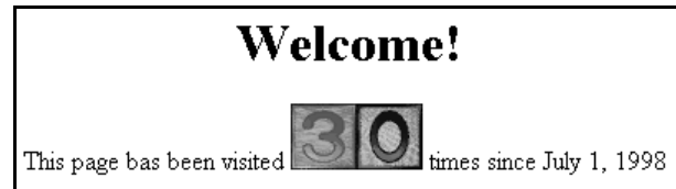
Figure 6 - Number of page visits shown by on-the-fly constructing HTML image references to images that exist as numbered GIF files, one per digit.
