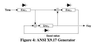
In the X9.17 generator the encryption step labelled  $Enc_1$  ensures that the timestamp is spread over 64 bits and avoids the threat of a chosen-timestamp attack (for example setting it to all-zero or all-one bits), the  $Enc_2$  step acts as a one-way function for the generated encryption key, and the  $Enc_3$  step acts as a one-way function for the seed value/internal state. The generator presented here replaces the keyed triple-DES
