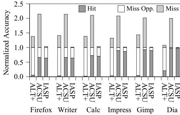
Figure 5: Prediction accuracy normalized to the total number of disk spin-ups without the buffer cache.
