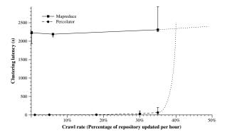
**Figure 7:** Median document clustering delay for Percolator (dashed line) and MapReduce (solid line). For MapReduce, all documents finish processing at the same time and error bars represent the min, median, and max of three runs of the clustering MapReduce. For Percolator, we are able to measure the delay of individual documents, so the error bars represent the 5th- and 95th-percentile delay on a per-document level.
