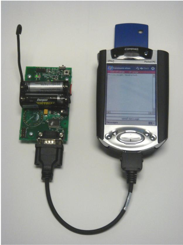
Figure 13: Mobile node with RFID reader
