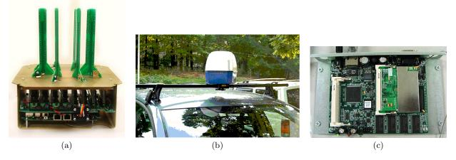
Figure 4: Hardware setup: (a) *MobiSteer* node – open; (b) *MobiSteer* node – in cover and mounted on a car; (c) embedded router platform for APs in controlled experiments.
