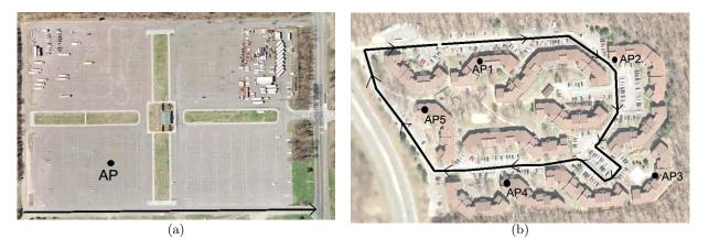
Figure 8: Two environments for the controlled experiments: (a) a large empty parking lot in the Stony Brook university campus, (b) a student apartment complex in the same campus. The black dots show the AP locations and the black arrow shows the driving route.
