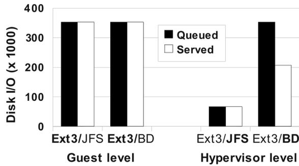
Figure 9: Disk I/Os under sequential read workload
