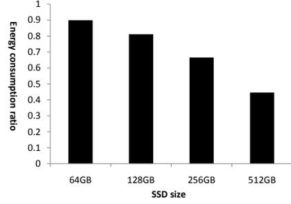
Fig. 1. Energy consumption ratio against the SSD size.
