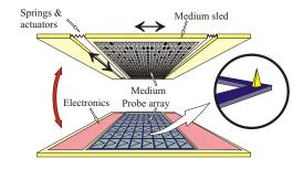
Fig. 1. A 3D view of a MEMS-based storage device. Two layers facing each other where the medium sled is attached to springs that suspend it over the probe array.
