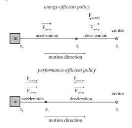
Fig. 2. The energy-efficient shutdown policy versus the performance-efficient one. The latter uses the actuators for acceleration.
