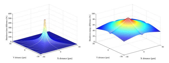
Fig. 3. Relative difference in shutdown time (*left*) and energy (*right*) between the performance-efficient (PE) policy and the energy-efficient (EE) policy calculated as  $\frac{t_{\rm EE} - t_{\rm PE}}{t_{\rm PE}}$  and  $\frac{E_{\rm PE} - E_{\rm EE}}{E_{\rm PE}}$ , respectively.
