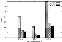
Energy Use of scp Encryption Cost by Cipher
