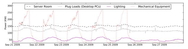
Figure 1: Detailed breakdown of the various power consumers inside the CSE building at UC San Diego [4], for a week in September 2009. Desktop computing equipment, which make up majority of the plug loads, and the IT equipment in the server rooms account for almost 50% to 80% of the base load of this building.
