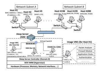
Figure 4: SleepServer implementation based on XEN.
