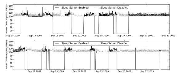
Figure 6: Comparing the Power Consumption for a Desktop PC with and without Sleep-Servers. For the first two weeks from August 31st - Sept 13th the user was not using SleepServer, while from Sept 14th to September 28th, SleepServer operation was enabled. Additionally, from Sept 22nd onwards the PC was set to automatically go to sleep within one hour of idleness.
