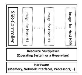
Figure 3: A example SleepServer serving a collection of host PCs (H1, ...H99). All resource sharing and access to the hardware is mediated by the SleepServer controller software module running on the SleepServer.
