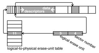
Figure 3: Translating a logical pointer into a physical address. The logical pointer consists of a logical erase unit (3 in the figure) and a sector number (4 in the figure). The logical-to-physical erase-unit table maps logical unit 3 to physical unit 11, which is the erase unit shown in the figure. The pointer stored in descriptor number 4 in erase unit 11 points to the address represented by the logical pointer.
