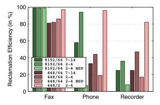
Figure 10: Reclamation efficiency under different device/file-system scenarios.
