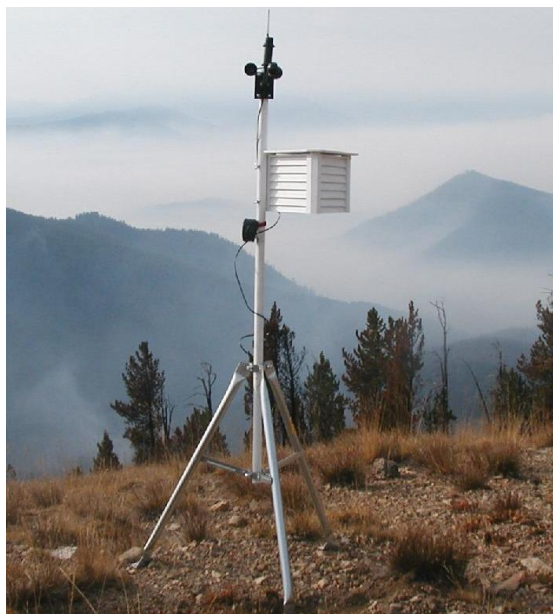
(a) An enclosure we built for our sensor nodes. The open bottom, vented ceiling, and slotted walls allowed the sensors to accurately record conditions.
