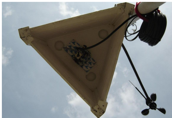
(b) Nodes were attached to the ceiling with industrial velcro. All sensors faced down towards the open bottom.
