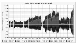
Figure 9: Graph produced 2000/09/21 showing campus traffic by network over the past 550 days.
