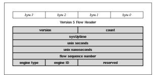
Figure 2: An image of Cisco's NetFlow V5 PDU header [McRobb].
