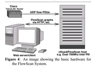
While FlowScan does not have strict platform requirements, most users who have successfully deployed it have dedicated either a SPARC machine running Solaris or Intel machine running GNU/Linux or BSD as a FlowScan system. Deploying on one of these platforms is also convenient because cflowd builds and runs on them as well, which allows one to co-locate FlowScan with cflowd so that both have access to the local disk. The fastest FlowScan machines appear to all be multi-processor Intel machines.
