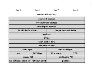
Figure 3: An image of Cisco's NetFlow V5 PDU entry [McRobb].
