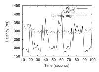
Figure 3: Using an STR to control workload shares in WFQ and C-WFQ. The graph depicts one of the workloads in the system. WFQ results in an unstable system that misses workload goals.
