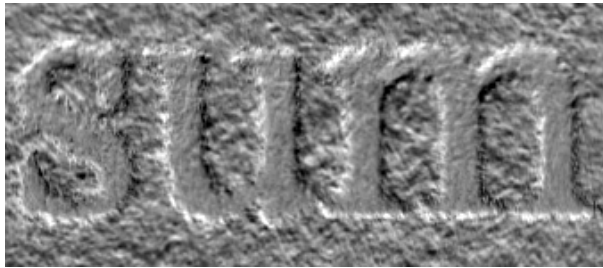
(b) Image depicting the surface texture as measured by two 1200 DPI scans. After only two scans, the geometry of the paper surface is clearly visible. The embossing effect of the text is actually the wax ink sitting on top of the paper surface.
