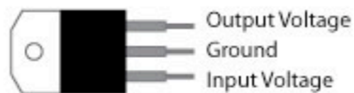
L7805 Positive +5V Voltage Regulator
