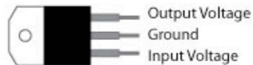
L7805 Positive +5V Voltage Regulator
