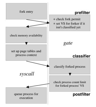
Figure 7: Control-flow of the fork gate
