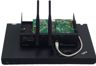
Figure 11: Experimental hardware setup of the UDSSS implementation, consisting of a Universal Software Radio Peripheral (USRP) and a Lenovo T61 ThinkPad.
