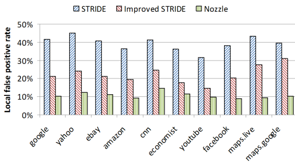
Figure 12: Local false positive rate for 10 benchmark web sites using NOZZLE and STRIDE. Improved STRIDE is a version of STRIDE that uses additional instruction-level filters, also used in NOZZLE, to reduce the false positive rate.
