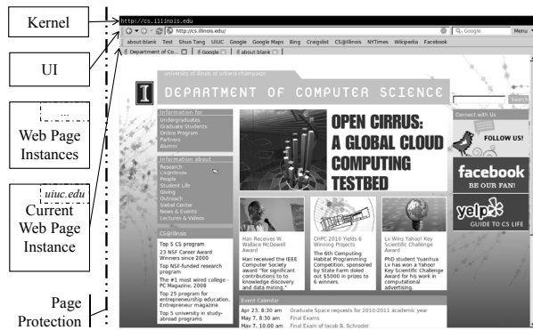
Figure 3: IBOS display isolation. This figure shows how IBOS divides the display into three main parts: a bar at the top for the kernel, a bar for browser chrome, and the rest for displaying web page content. The IBOS kernel enforces this isolation using page protections and without relying on a window manager.
